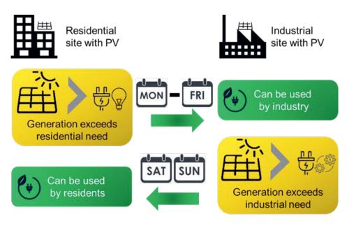
Figure 4: Example of an energy community with industrial and residential sites (Source: Siemens)
