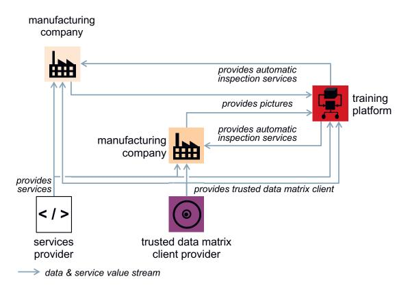
Figure 9: Trusted Data Matrix for algorithm training for automatic quality inspection with multiple data sources
