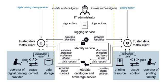
Figure 16: Technical perspective of use case 'Trusted data sharing of digital printing drawings'
