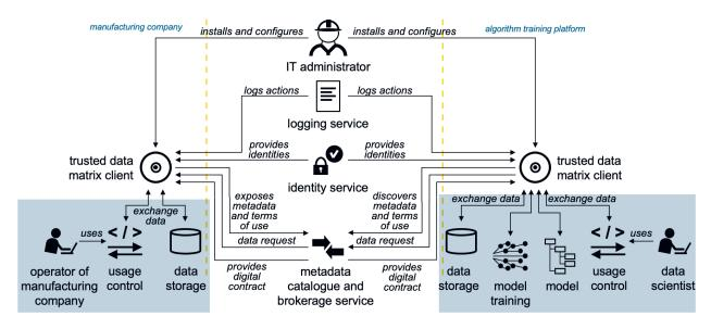
Figure 15: Technical perspective of use case 'Trusted model training with multiple data sources'
